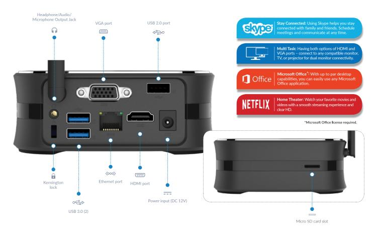
The HDMI along with the VGA port remain in the middle. A Micro SD card connector is integrated providing up to 128GB of storage for any application. Not to forget, the Byte Plus comes with an Ethernet port which allows you to plug in an Ethernet cable directly into your Mini PC for uninterrupted internet service.
